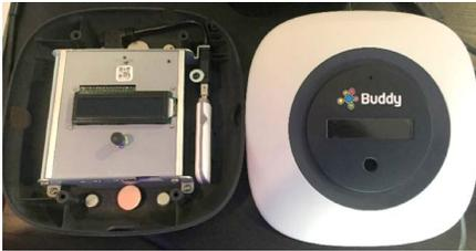
Open the top cover of the Buddy Ohm device and Install the antenna to the Ohm.
